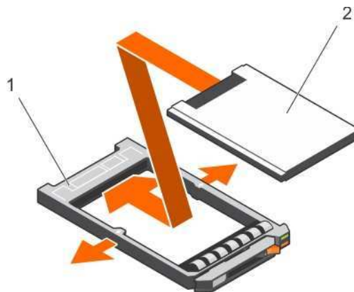
Figure 40. Installing a 1.8-inch hard drive into a hard drive carrier
