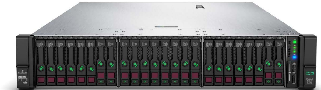
24 SFF (incl 12 NVMe SSDs) hot-plug drive model
